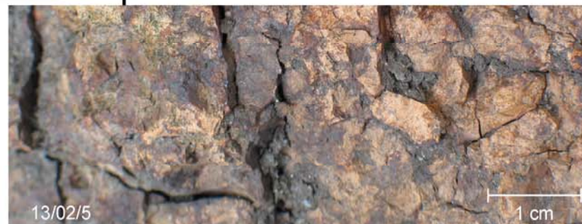
blast furnace reduction slags with cast iron nodules from Forno di Lemie and Richiaglio (Viù)
