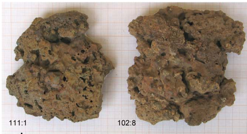
thermo-altered wall fragments of Forno di Lemie blast furnace
