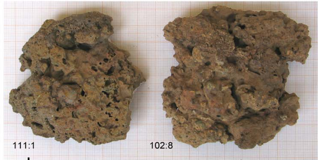
thermo-altered wall fragments of Forno di Lemie blast furnace
