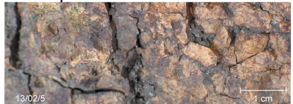
blast furnace reduction slags with cast iron nodules from Forno di Lemie and Richiaglio (Viù)
